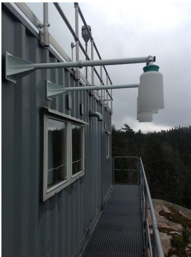
*Figure 5: Photograph of the sampling inlet used for the measurements at the Birkenes Observatory.*
