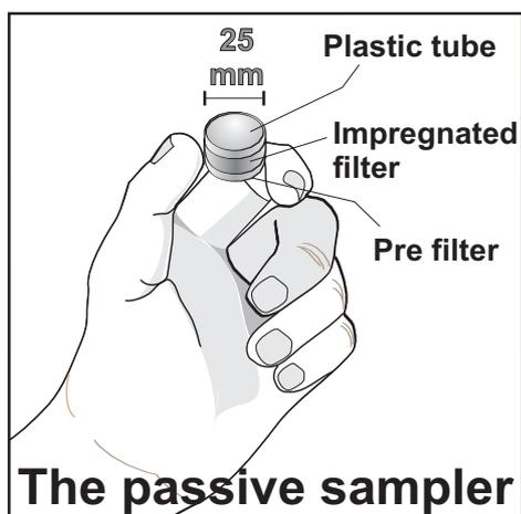
A sensitive diffusion sampler for sulphur dioxide (SO<sub>2</sub>) and nitrogen dioxide (NO<sub>2</sub>) in ambient air has been used in several investigations to undertake a screening of the spatial concentration distribution.
