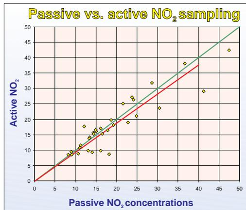
*The integrated passive sampling of SO<sub>2</sub> and NO<sub>2</sub> is well correlated with available active sampling methods.*
