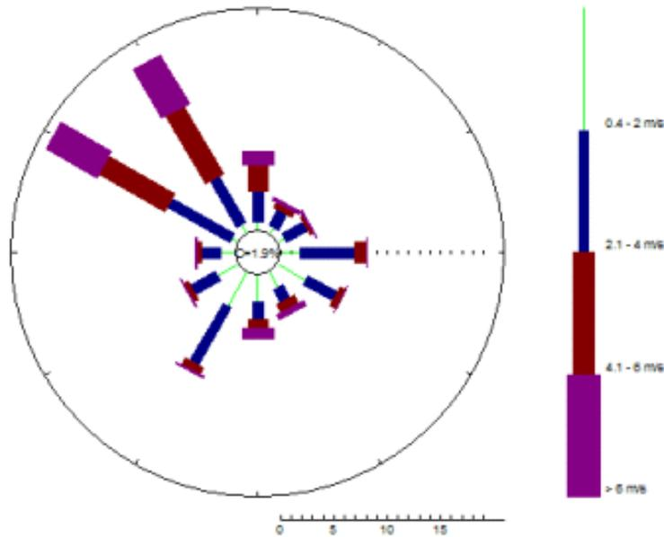
Figure 5: Wind rose for the modelled period. The meteorological station was placed between the Maqta and Mussafah Bridges in Abu Dhabi city.
