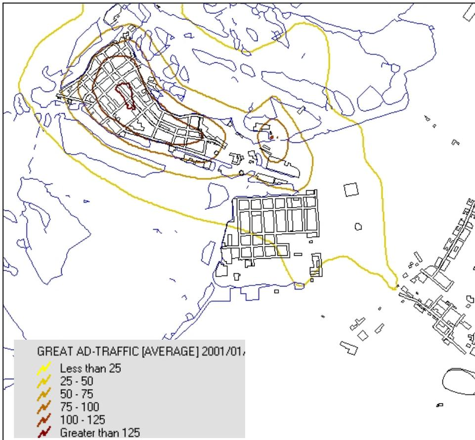
Figure 8: Average NO<sub>2</sub> (top figure)/NO<sub>x</sub> (bottom figure) concentrations (μg/m<sup>3</sup>) from traffic and industrial emissions in Abu Dhabi city for a 6-month period.
