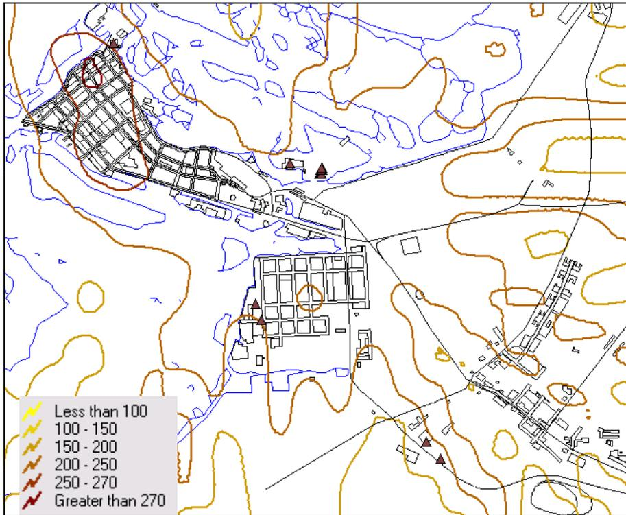
Figure 9: Typical maximum one hour average NO<sub>2</sub> concentrations ( $\mu\text{g}/\text{m}^3$ ) from traffic and industrial emissions in Abu Dhabi city.
