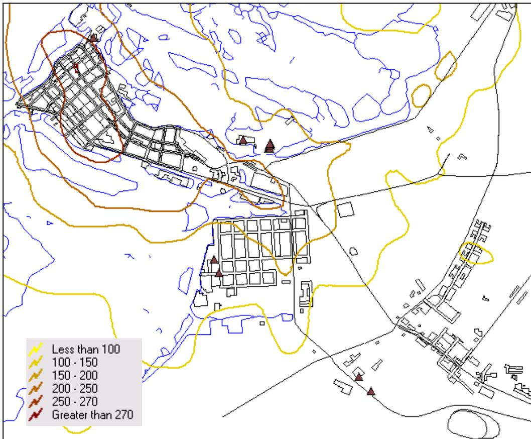
Figure 7: Typical maximum one-hour average NO<sub>2</sub> concentrations (µg/m<sup>3</sup>) from traffic emissions in Abu Dhabi city.
