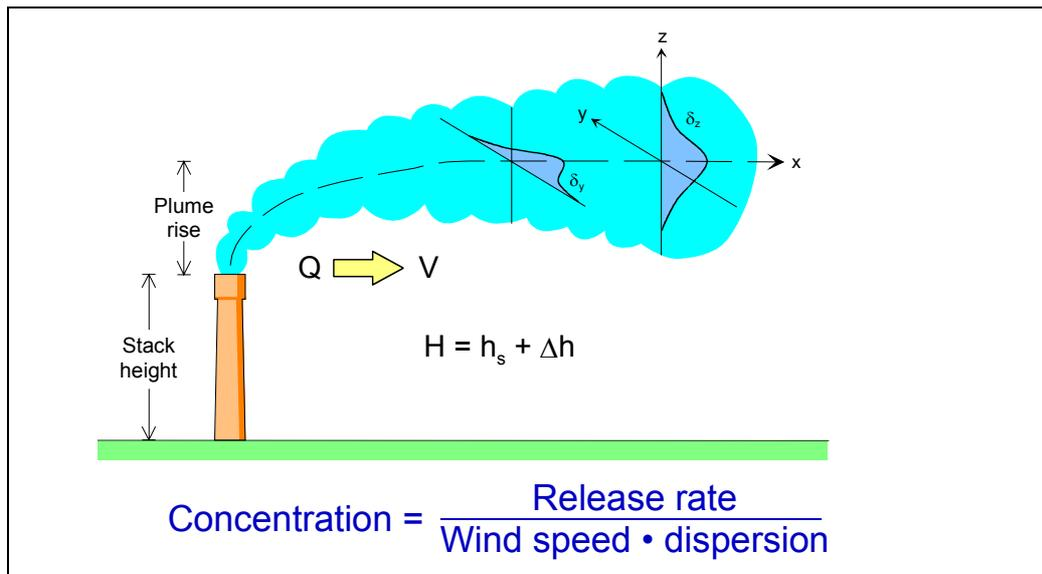
Figure 1: The concept of the Gaussian plume model.
