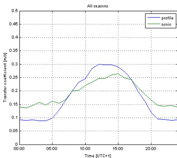
Figure 22: Average diurnal cycle of the transfer coefficient in Hurdal over the measurement years calculated from profile assumptions according to Mikkelsen et al. (2000) or determined with sonic data.
