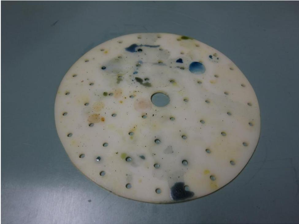
Figure 15: Dissolved copper in DEA solution of high concentration having run off a copper sample.
