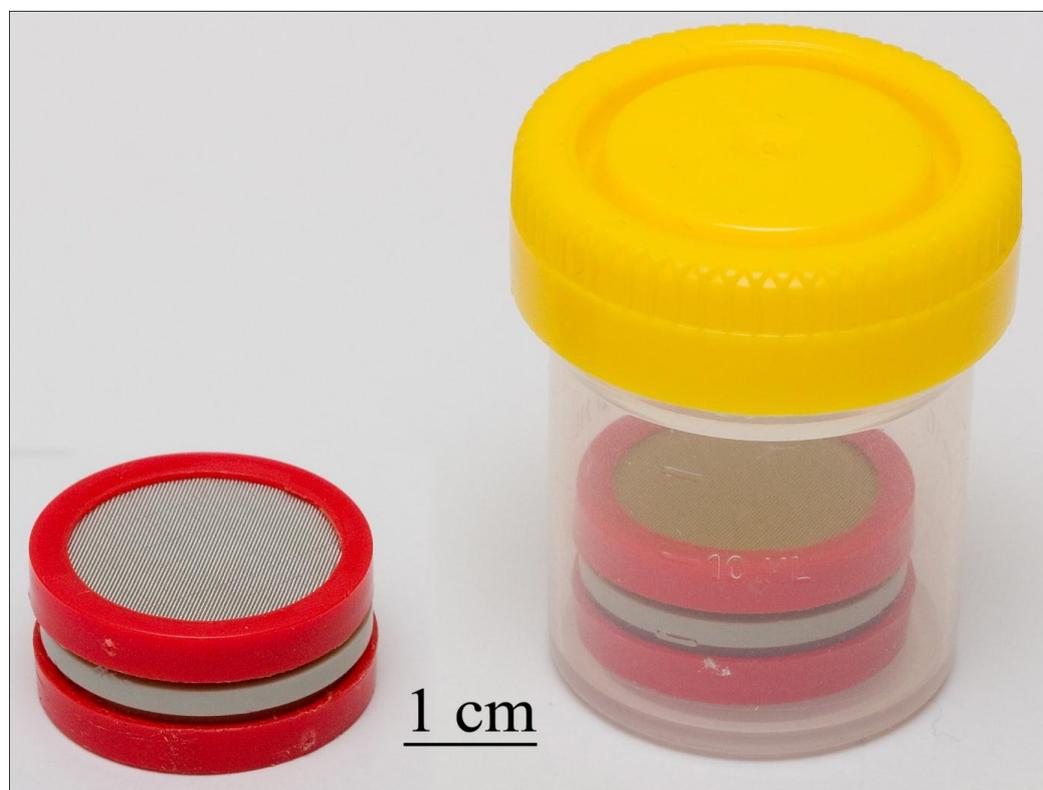
Figure 6: *Passive  $\text{SO}_2$  sampler.*
