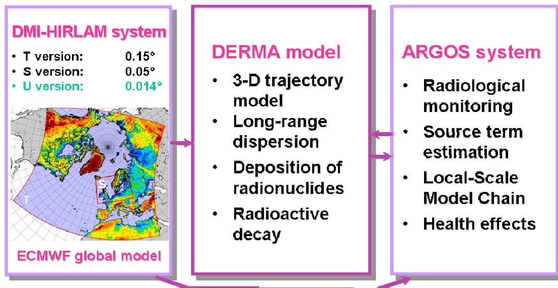
Figure 7.1: Structure of the Danish nuclear emergency modelling system.
