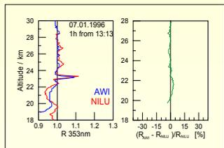
**Fig. 1:** Backscatter ratio  $R$  of the 353 nm lidar measurement at ALOMAR on January 07, 1996, analysed by *AWI* (blue) and *NILU*(red) [left]. Deviation of the algorithm results [right].
