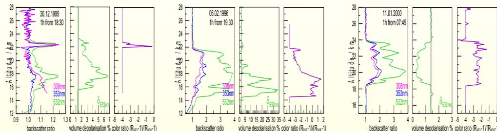
**Fig. 4a, b, and c:** Examples for December 30, 1995, February 06, 1996 and January 11, 2000. For each day the backscatter ratio for 308 nm using *NILU*  $O_3$  correction, as well as for 353 nm and 532nm from *AWI* aerosol algorithm, the volume depolarisation at 532 nm from *AWI* aerosol algorithm, and the Color ratio  $C = (R_{353-1}) / (R_{308-1})$  from *NILU*  $O_3$  correction algorithm are shown.
