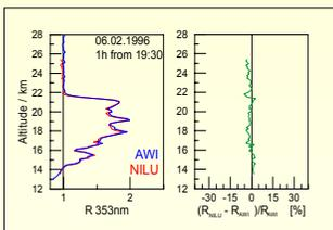
**Fig. 2:**  $R$  at 353 nm of the Ny-Ålesund lidar measurement on February 06, 1996, analysed by *NILU* (red) and *AWI* (blue).
