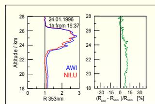
**Fig. 3:**  $R$  at 353 nm of the lidar measurements at ALOMAR on January 24, 1996 analysed by *AWI* (blue) with fitting range 26.5–27.6 km and *NILU* (red).
