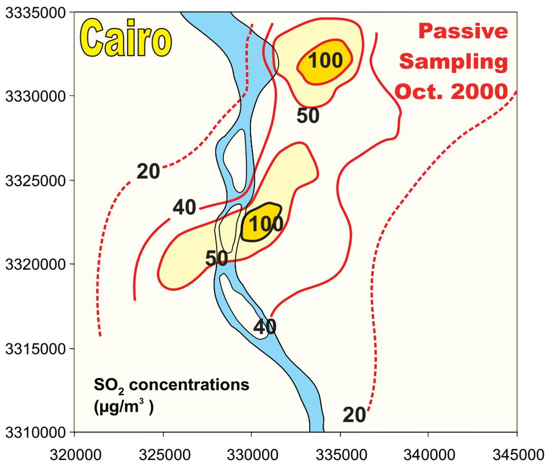
Figure 2: SO<sub>2</sub> concentrations measured by passive samplers in Cairo, 14-28 October 2000.
