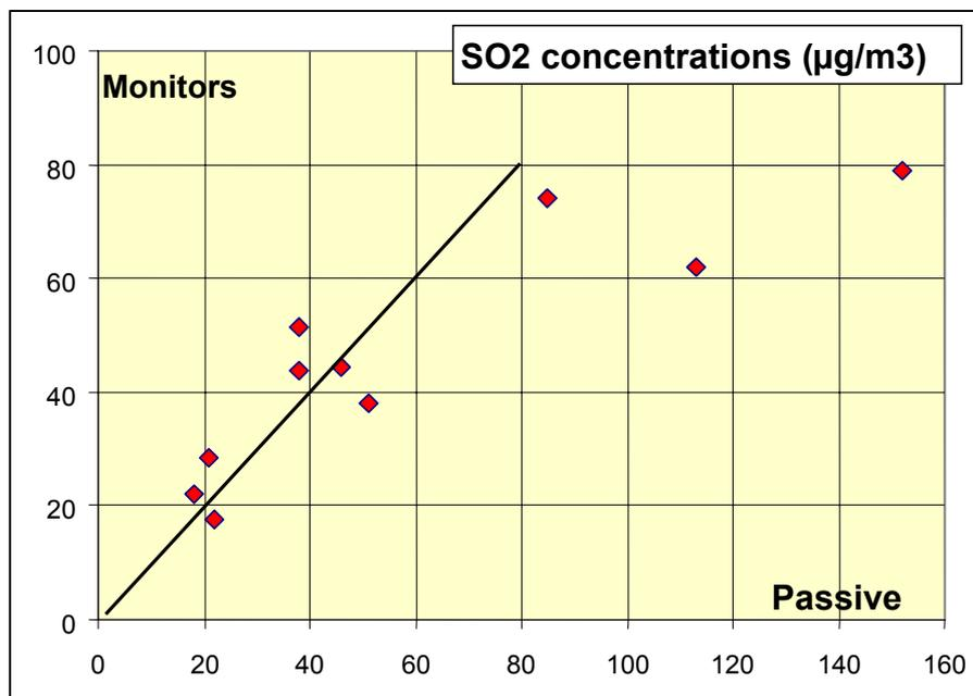
Figure 4: SO<sub>2</sub> concentrations from passive samplers versus SO<sub>2</sub> by monitors based on measurements performed in Cairo from 14 to 28 October 2000.
