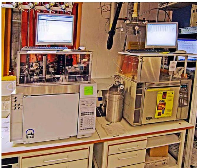
Figure 55: The new Gas Chromatograph for Methane and Nitrous Oxide measurements (left) side by side with the old system for Methane measurements.
