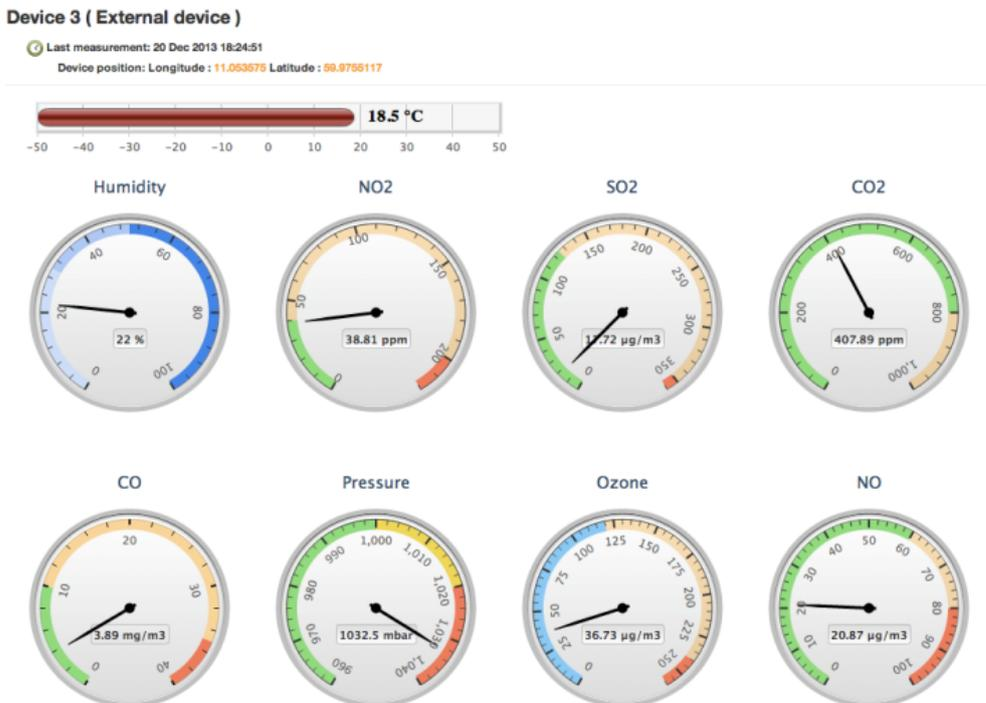
Figure 10: Examples of real-time sensor information from the Dunavnet sensor platform
