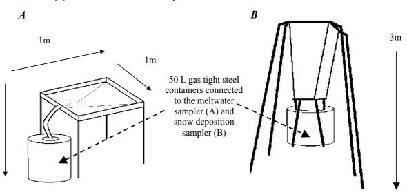
Figure 2: Snow deposition - and melt water collectors used for sampling of snow and melt water at Bjørnøya.
