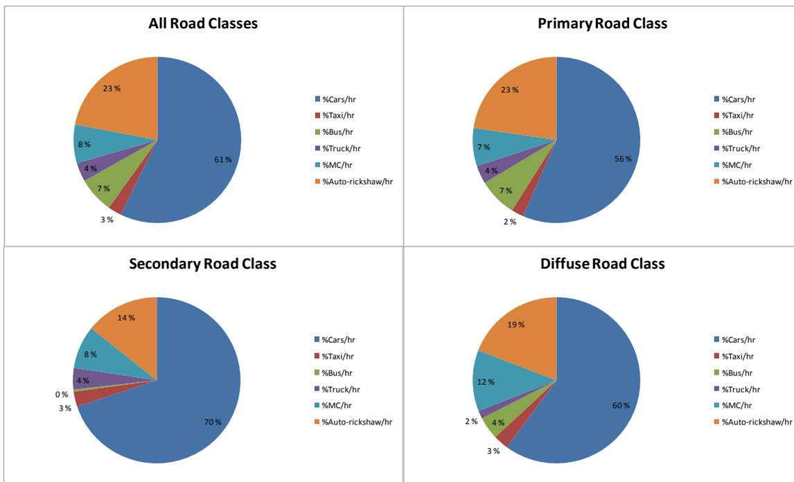
Figure 44: Vehicle class distributions for each road class.
