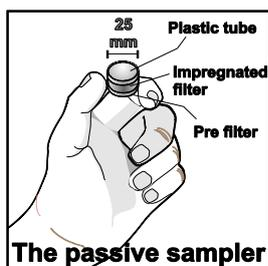
Figure 6: Illustration of passive sampler.
