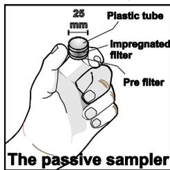
These samplers have been used by NILU in a number of studies (Hak, 2010; Hak and Sivertsen, 2010). For sampling of gases they include an impregnated filter inside a small plastic tube. To avoid turbulent diffusion inside the sampler, the inlet is covered by a thin porous membrane filter. Gases are transported and collected by molecular diffusion.
