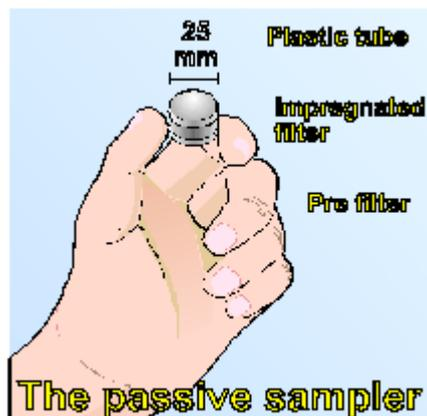
A sensitive diffusion sampler for sulphur dioxide ( $\text{SO}_2$ ) and nitrogen dioxide ( $\text{NO}_2$ ) in ambient air has been used in several investigations to undertake a screening of the spatial concentration distribution.
