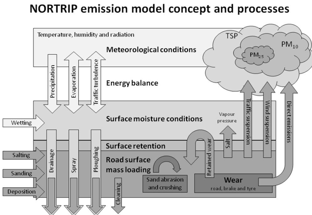
Figure 1: NORTRIP model concept showing the full model processes. Sand abrasion and crushing, as well as windblown suspension, are not included in the current application.
