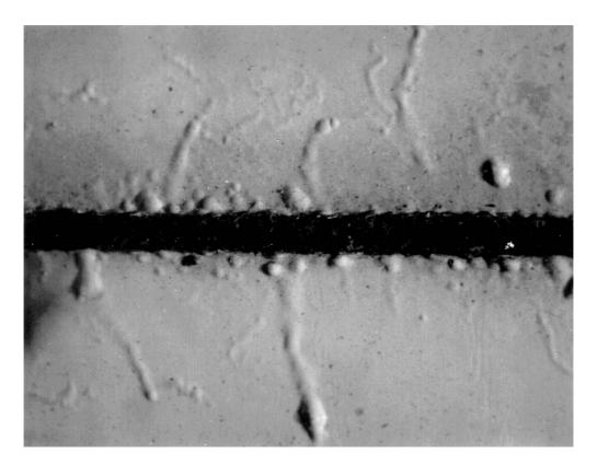
*Figure 2: Filiform attack from the cut on alkyd painted panels at site Lincoln Cathedral.*
