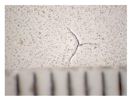
*Figure 5:* The paint substrate with cracks after four years of exposure at site 16 Venice.
