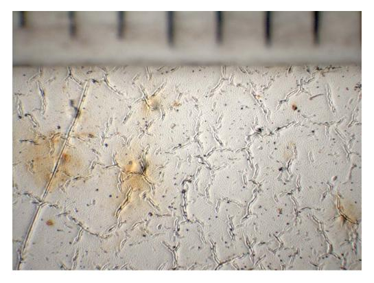
*Figure 3:* The paint surface after four years of exposure at site 43 Tel Aviv.
