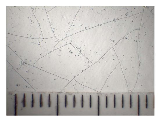
*Figure 4:* The paint substrate after four years of exposure at site 37 Dorset, Canada.
