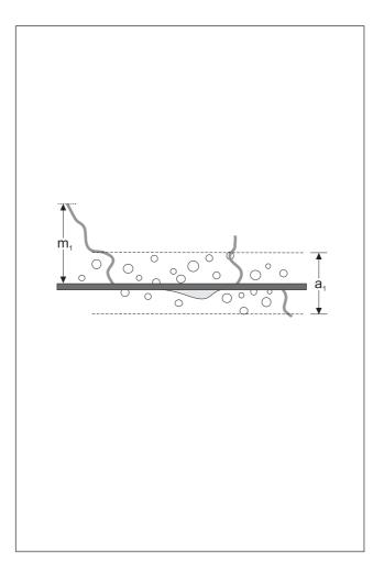
*Figure 1:* Illustration of evaluation for spread from the cut and filiform corrosion on the test panels.
