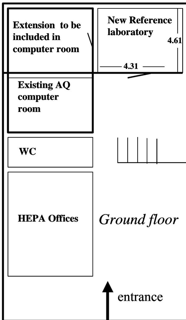
The space for the new Reference Laboratory was inspected. The location is in the first floor of the HEPA building. The size of the room is 4.60m x 4.31 m and the height is 2.15 at the lowest point and about 3.5 m at the highest point.
