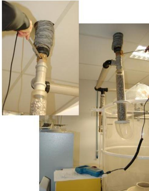
Figure 11: Flow measurements at the outlet of the fog chamber.
