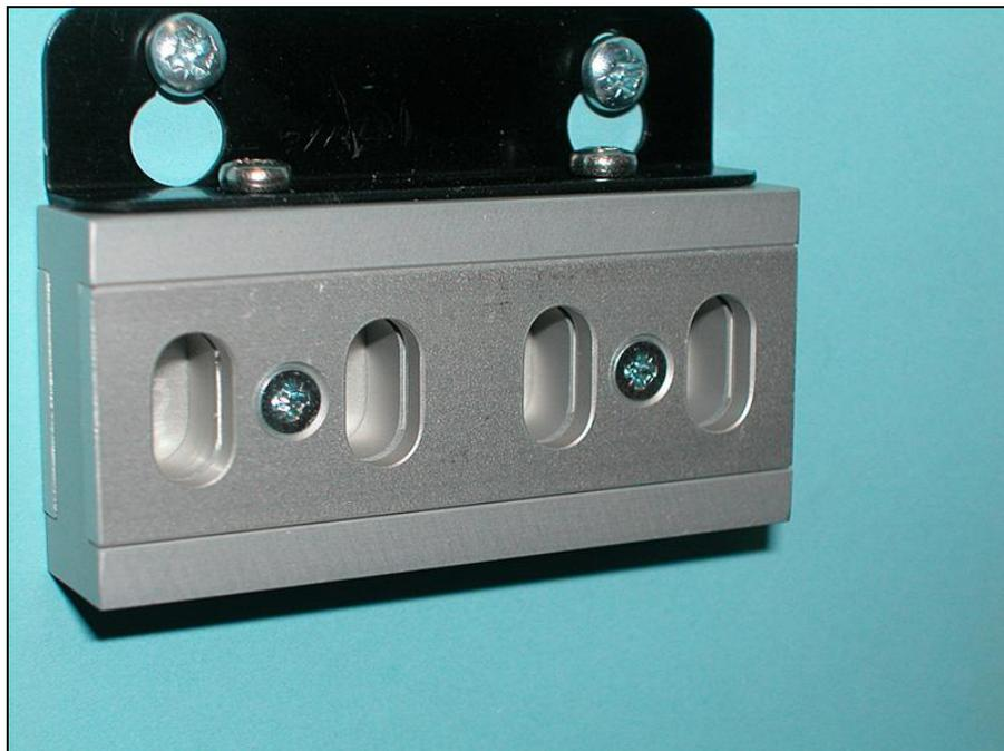
*Figure 2.11: EWO-G dosimeter holder for analysis in laboratory.*
