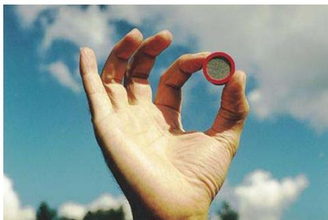
One of the internationally recognised sampler was developed by the Swedish Environmental Research Institute (IVL) and has been used in several cases by NILU. The sampler includes an impregnated filter inside a small plastic tube.
