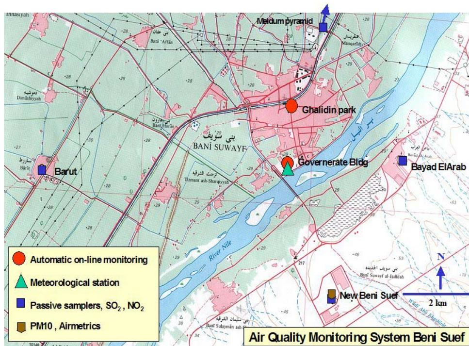
Figure 1: The air quality monitoring network proposed for Beni Suef.
