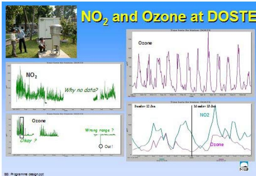
NO<sub>2</sub> and ozone at DOSTE worked properly for a short period in January 2003. The present ozone measurements show a range, which is too small. The instrument must be calibrated.
