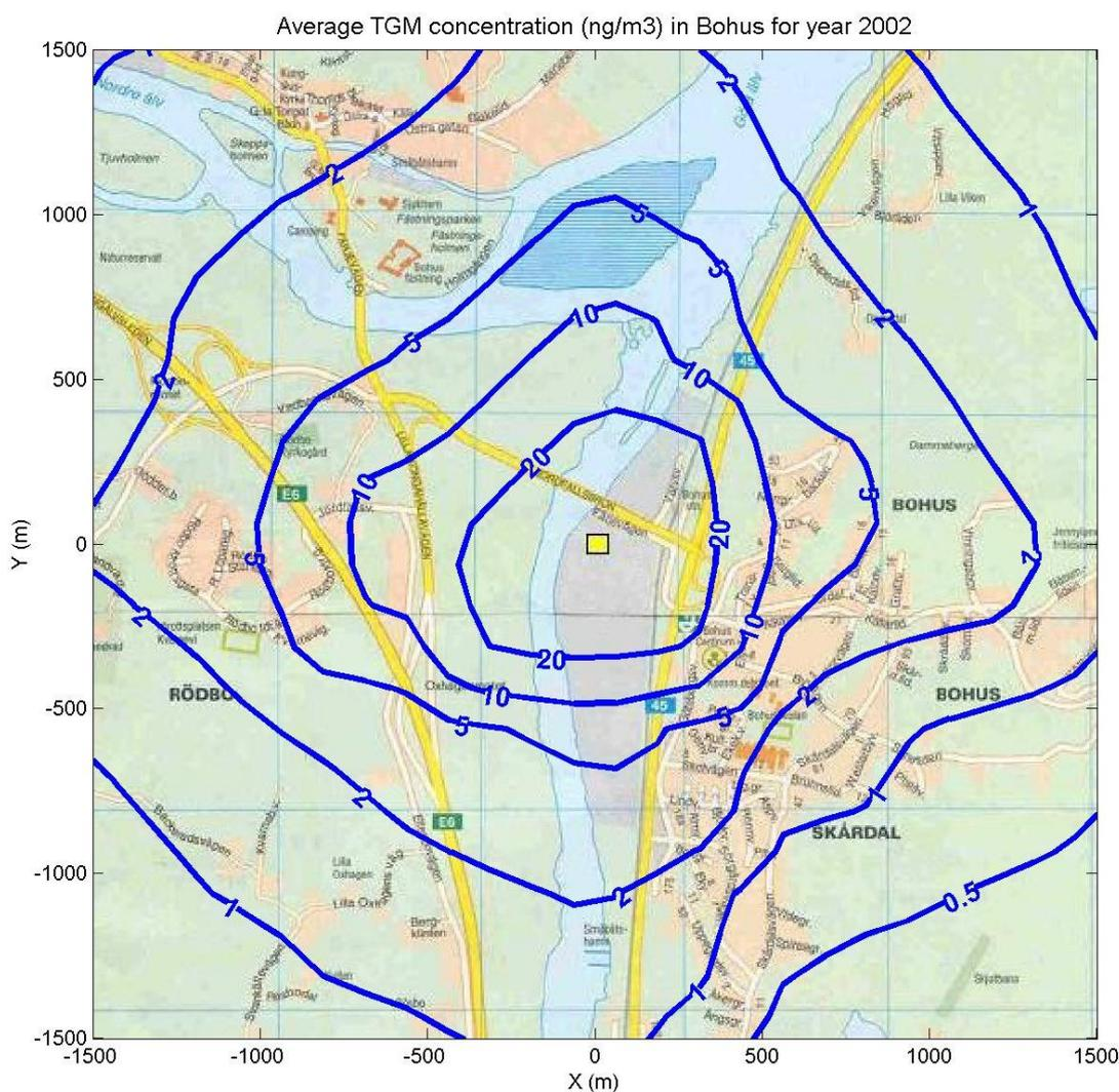
Figure 7. Average annual TGM concentration (ng/m<sup>3</sup>) for the Bohus plant in Sweden, calculated for the year 2002. Contours are in uneven intervals of 0.5, 1, 2, 5, 10, 20 and 50. The yellow square shows the position of the plant. Background concentrations are not included.
