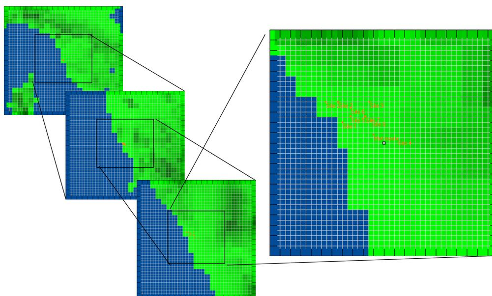
Figure 1. Showing the 4 nested meteorological grids used in the TAPM simulations for Rosignano.
