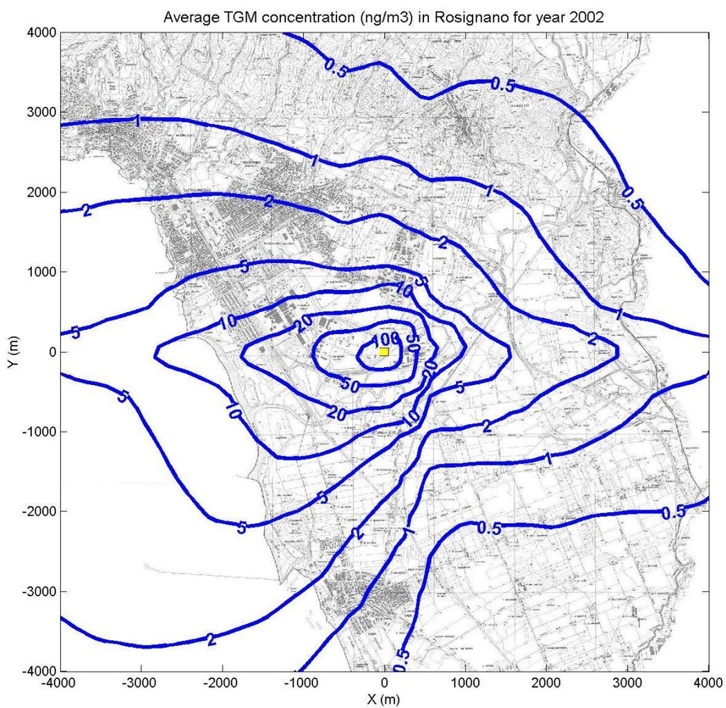
Figure 5. Average annual TGM concentration (ng/m<sup>3</sup>) for the Rosignano plant in Italy, calculated for the year 2002. Contours are in uneven intervals of 0.5, 1, 2, 5, 10, 20, 50, 100 and 200. The yellow square shows the position of the plant. Background concentrations are not included.
