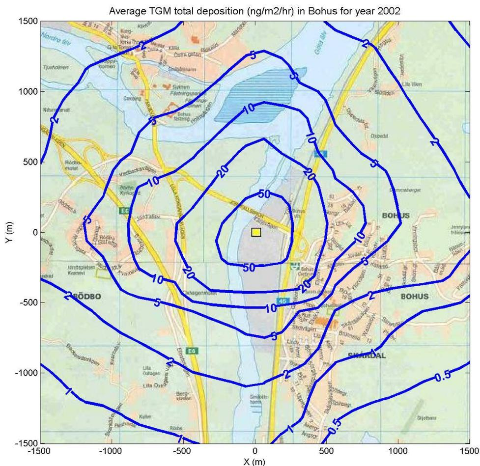
Figure 13. Annual average mercury dry deposition (top left), wet deposition (top right) and total deposition rate (ng/m<sup>2</sup>/hr) for the Bohus plant in Sweden, calculated for the year 2002. Contours are in uneven intervals of 0.5, 1, 2, 5, 10, 20, 50 and 100. The yellow square shows the position of the plant.
