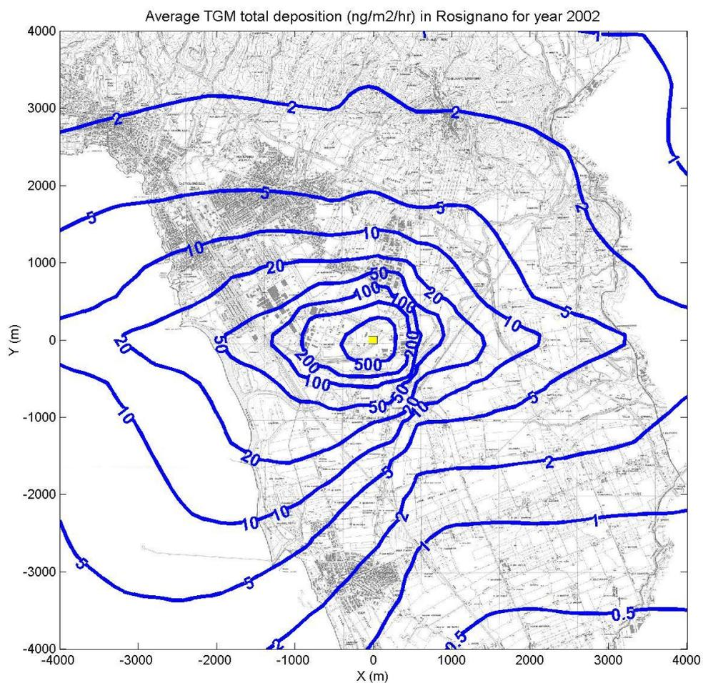
Figure 11. Annual average mercury dry deposition (top left), wet deposition (top right) and total deposition rate (ng/m<sup>2</sup>/hr) for the Rosignano plant in Italy, calculated for the year 2002. Contours are in uneven intervals of 0.5, 1, 2, 5, 10, 20, 50, 100, 200 and 500. The yellow square shows the position of the plant.
