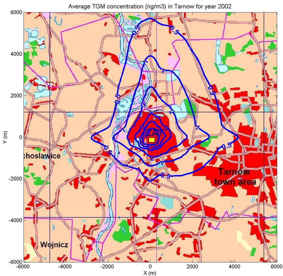
Figure 6. Average annual TGM concentration (ng/m<sup>3</sup>) for the Tarnow plant in Poland, calculated for the year 2002. Contours are in uneven intervals of 0.5, 1, 2, 5, 10, 20 and 50. The yellow square shows the position of the plant. Background concentrations are not included.
