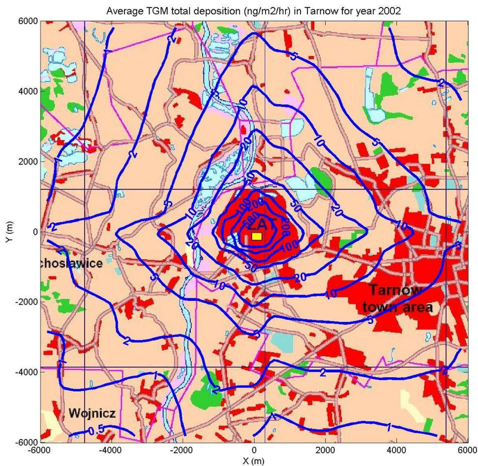
Figure 12. Annual average mercury dry deposition (top left), wet deposition (top right) and total deposition rate (ng/m<sup>2</sup>/hr) for the Tarnow plant in Poland, calculated for the year 2002. Contours are in uneven intervals of 0.5, 1, 2, 5, 10, 20, 50, 100, 200 and 500. The yellow square shows the position of the plant.
