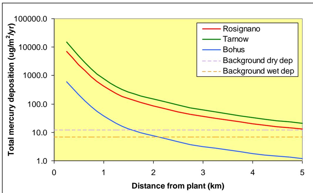
Figure 13. Average annual mercury deposition rate ( $\mu\text{g}/\text{m}^2/\text{yr}$ ) for all 3 plants, calculated for the year 2002, and shown as a function of distance from the plant. The vertical scale is shown as logarithmic.
