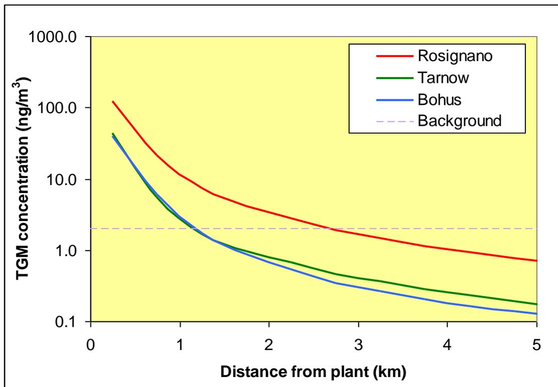
Figure 8. Average annual TGM concentration ( $\text{ng/m}^3$ ) for all 3 plants, calculated for the year 2002, and shown as a function of distance from the plant. The vertical scale is shown as logarithmic.
