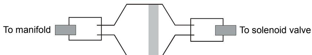
*Figure 2: Sintered glass filter in a glass bulb.*
