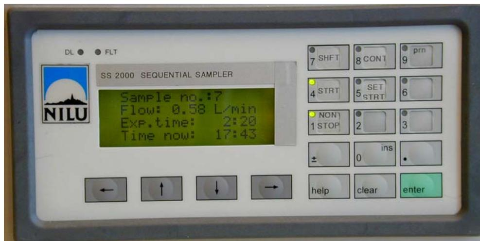
Figure A.2: Operator panel layout.
