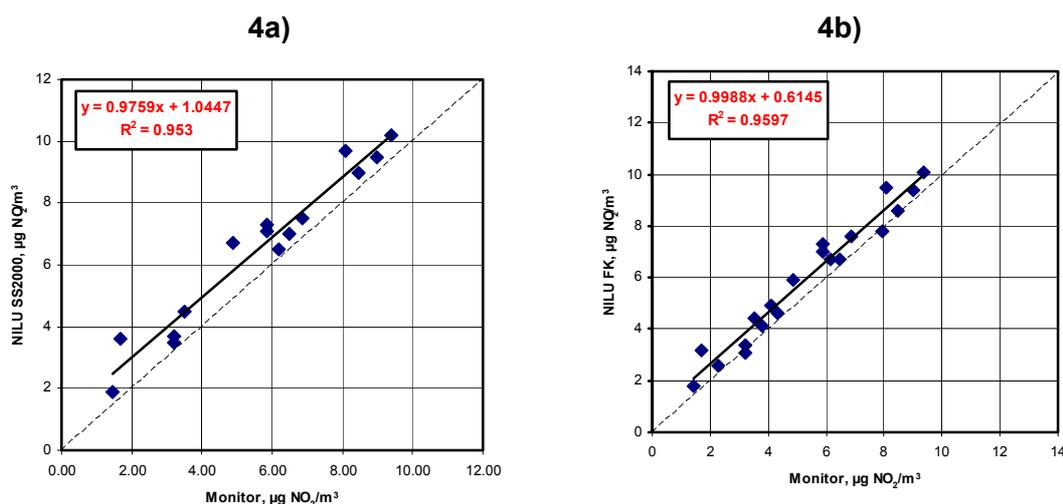
Figure 4: Correlation between: a) NILU SS2000 and monitor, and b) NILU FK and NO<sub>x</sub>-NO monitor
