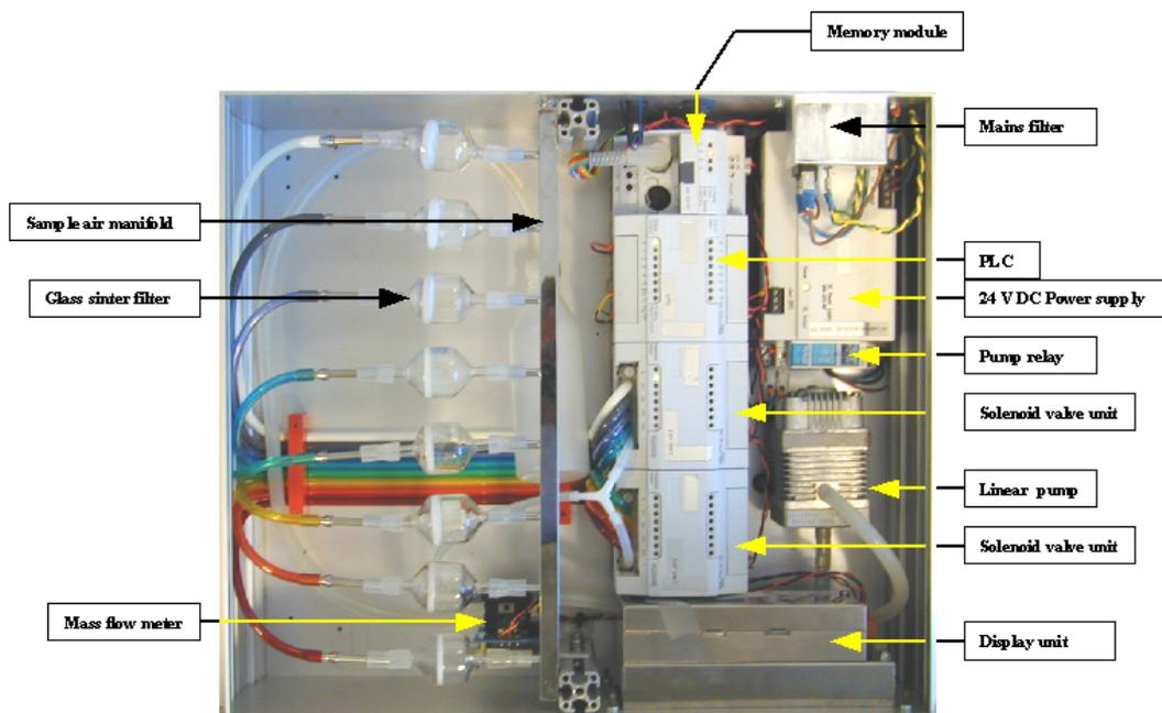
Figure A. 1: Instrument layout (lid removed).
