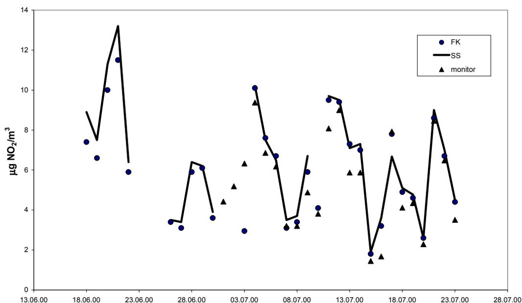
Figure 5: Comparison of NO<sub>2</sub> measurements using NILU-FK, SS2000 and monitor
