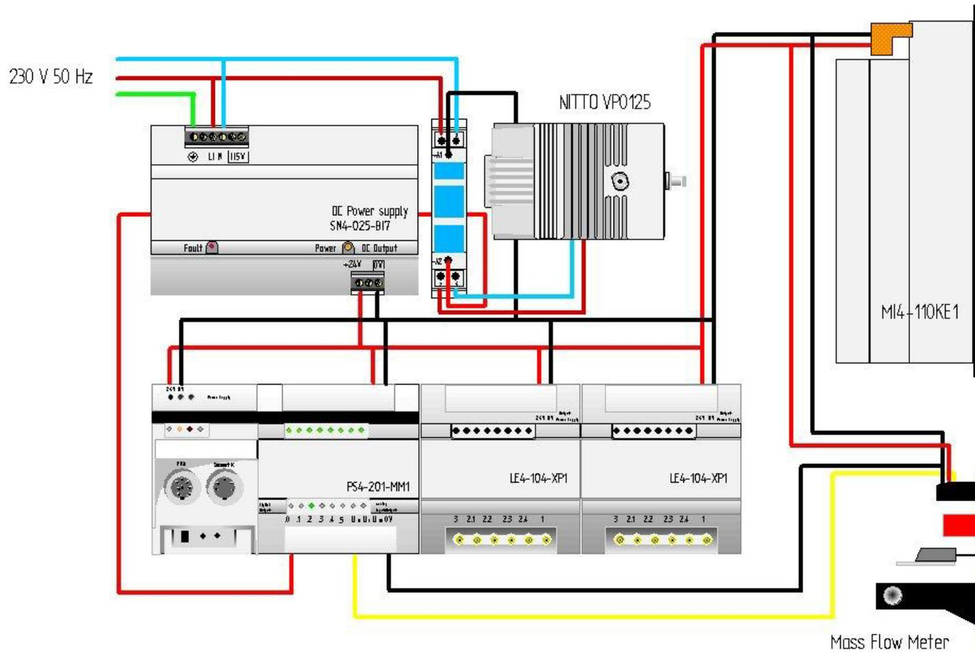
Figure C.1: Wiring diagram for NILU SS2000.
