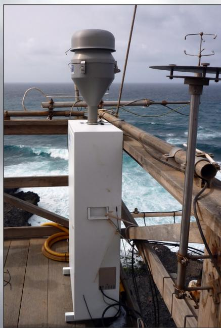
Figure 1: The active high-volume air sampler at CVAO.
