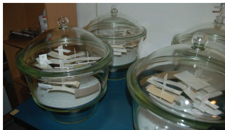
Paper samples are exposed to organic acids in the laboratory at NILU.
