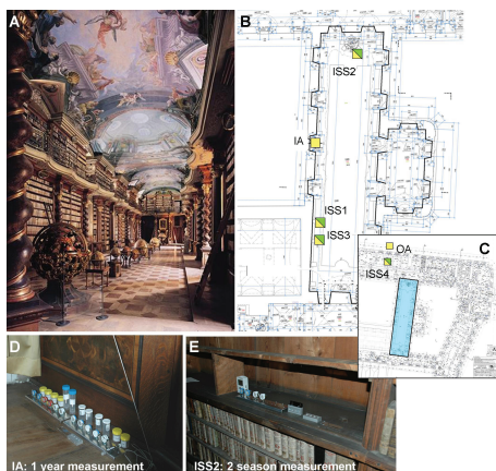
Figure 1: A: Baroque Hall of the National Library (Prague). B and C: Sampling locations; yellow square: locations of year measurement campaign; yellow/green squares: locations of two-seasonal measurement campaigns. Blue area in C: Baroque Hall. D and E: passive diffusion samplers and dosimeter.
