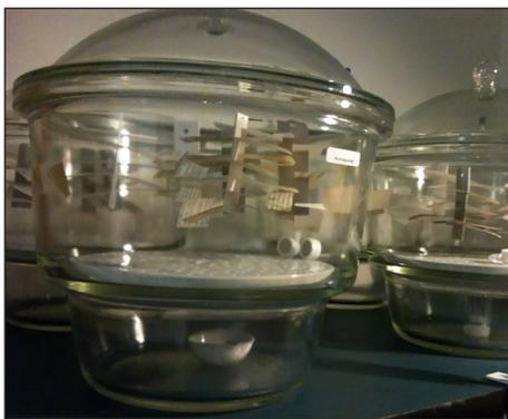
Fig. 3. Accelerated ageing of cellulosic materials exposed to acetic acid in the laboratory at NILU.
