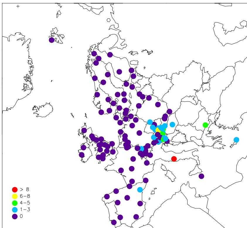
*Figure 1.4: Number of exceedances of the threshold value of 180 µg/m<sup>3</sup>. (Unit: number of days).*
