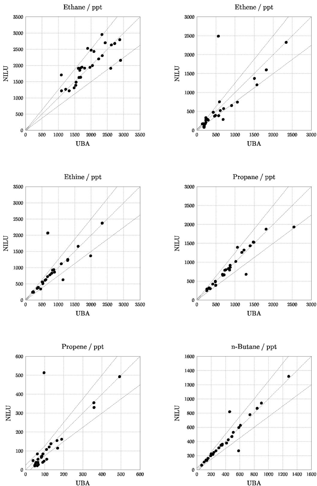
Figure 2: Scatter-plots of hydrocarbon parallel samples at Waldhof analysed by UBA and NILU. The slope-1-line and the DQO-limits (max ( $\pm 25\%$ ,  $\pm 25$  ppt)) are indicated by dashed lines.
