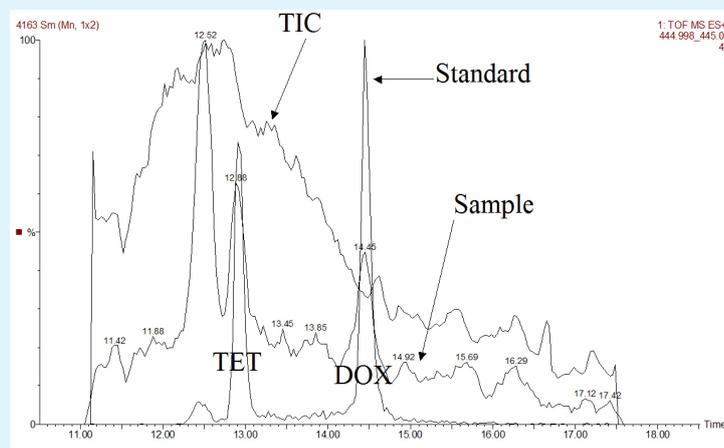
Figure 3: Chemical analysis of a STP sludge sample containing 487 ng/g (ww) Tetracycline (TET) and 242 ng/g (ww) Doxycycline (DOX).
