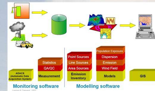
Figure 2: The AQM System [Laupsa & Fløisand, 2005]
