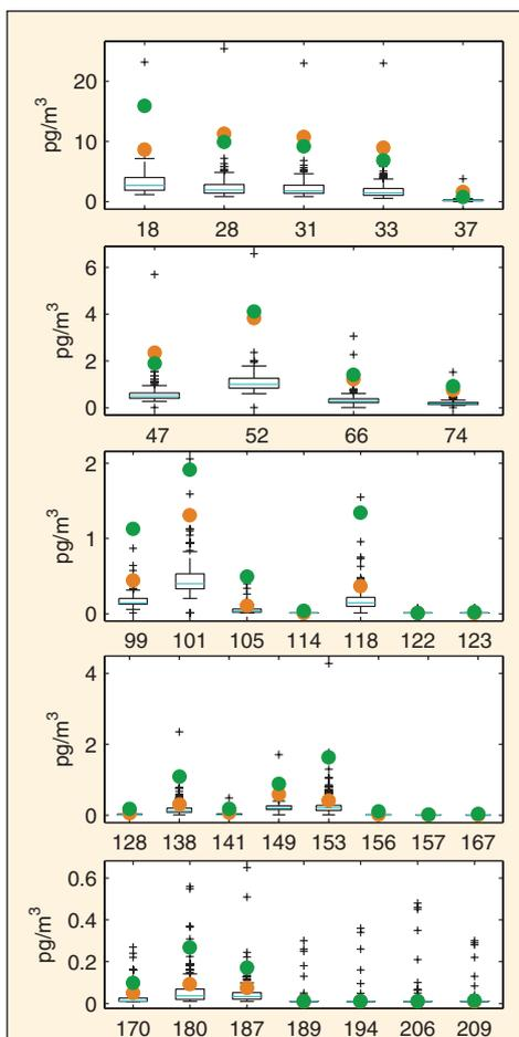
Figure 3: Box and whisker plots showing the frequency distributions of all PCB congeners [ $\text{pg}/\text{m}^3$ ] sampled at the Zeppelin station during the period from January 2002 to May 2006. The line shows the median, the box delineates the 25 and 75 percentiles, the whiskers are drawn at the 1.5 folded inter quartile range and the crosses mark outliers. The orange dots indicate the sample from 26 to 28 July 2004, the green dots indicate the sample from 1 to 3 May 2006.
