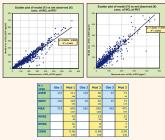
The adjusted model based on data assimilation no longer systematically overpredicts  $\mathrm{NO}_{\mathrm{X}}$  concentrations as shown at the independent stations 1 and 3
