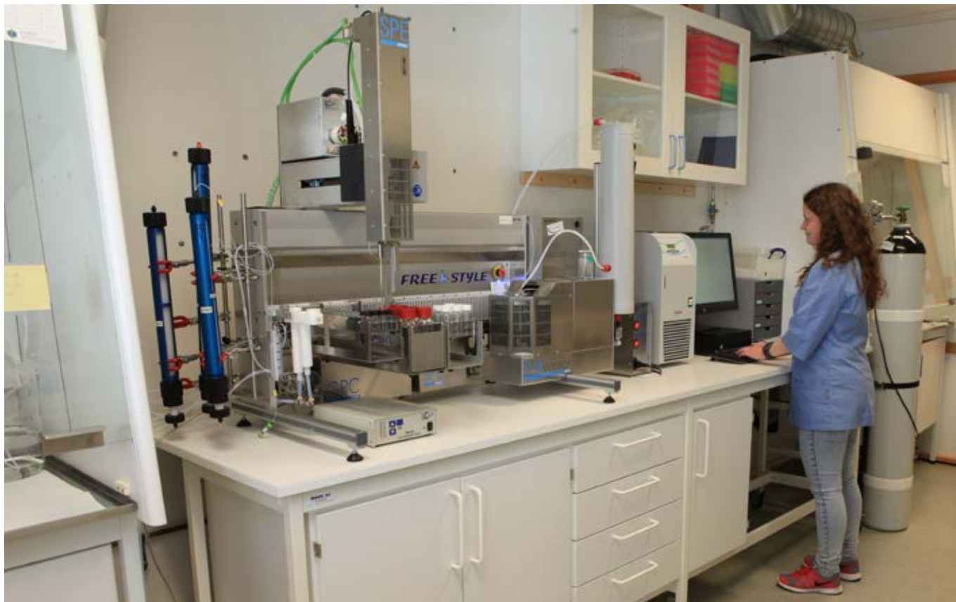
Silje Eltvik Thomassen from NILU's organic analysis lab starts a purifying process on the new robot from the PC. Photo: Ingunn Trones, NILU
