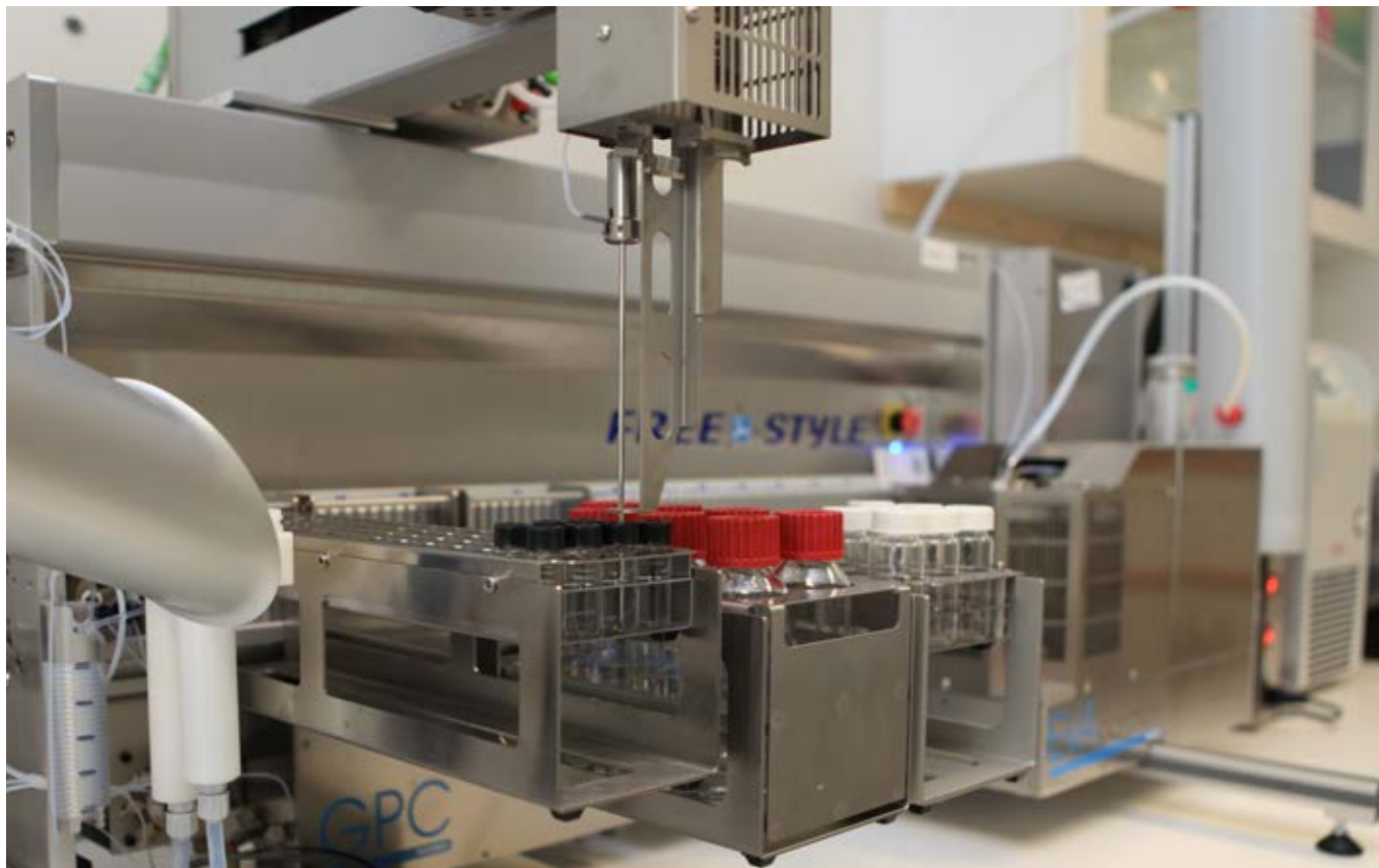
Some trays with extracted samples are inserted into the robot. The arm has moved and is ready to collect the sample. Photo: Ingunn Trones, NILU
