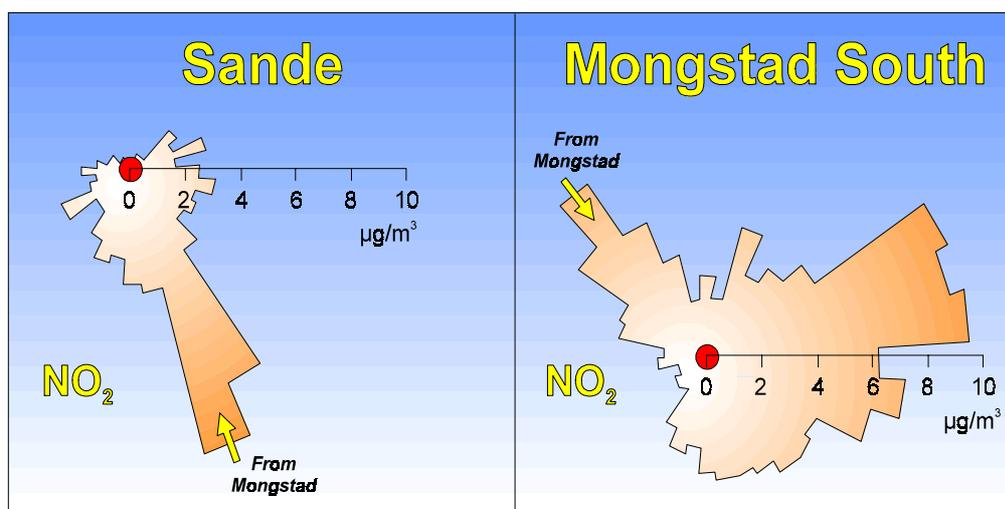
Figure 12.3: "Concentration rose", (Breuer diagram) established for two measurement sites at an oil refinery.
