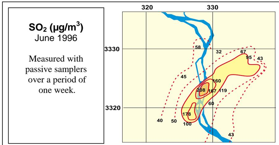
Figure 12.7: SO<sub>2</sub> concentration distribution for Cairo, based upon one week measurements with passive samplers, June 1996.
