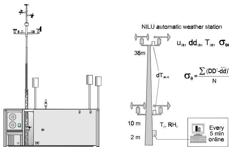
A complete air quality monitoring station consists of a set of monitors and samplers covering the relevant indicators for the specific site. The instruments are normally placed in an air-conditioned shelter, with telephone communication links to a central computer. For data retrieval and data quality assurance, see next chapter.
