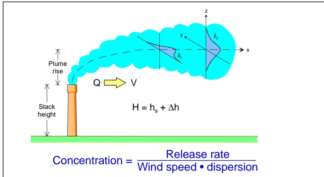
Table 10.1: The concept of the Gaussian plume model.
