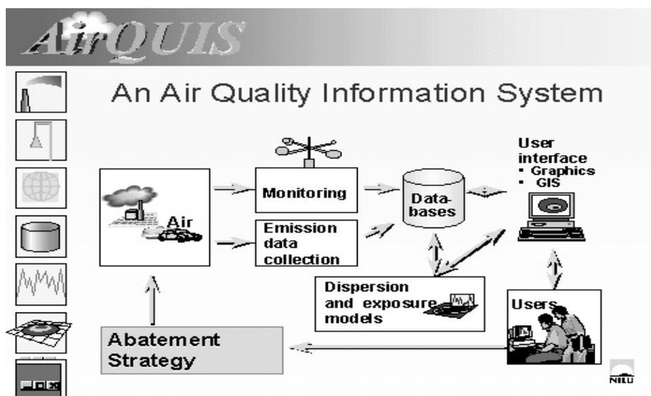
Figure 3.1: The principal structure of a modern environmental monitoring and information system.
