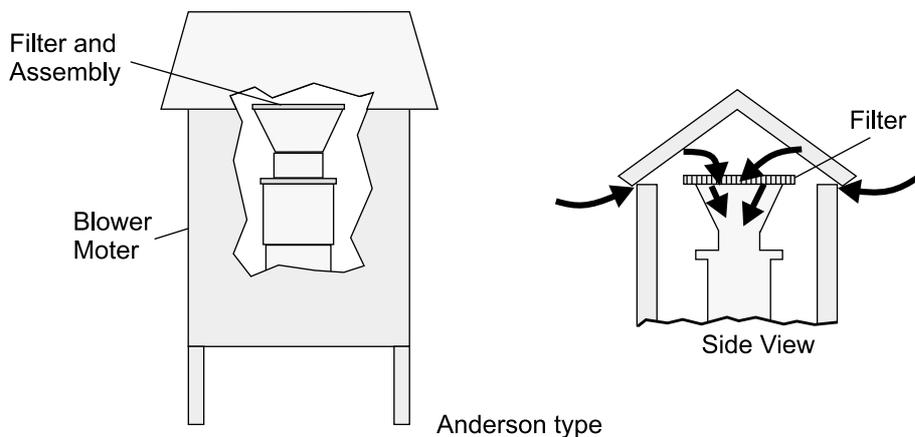
The covered housing protects the glass fibre filter from wind and debris, and from the direct impact of precipitation. The hi-vol collects particles efficiently in the size range of 0.3-100 micrometers. The mass concentration of total suspended particles (TSP) is expressed as µg/m<sup>3</sup> for sampling times of usually 24 hours.
