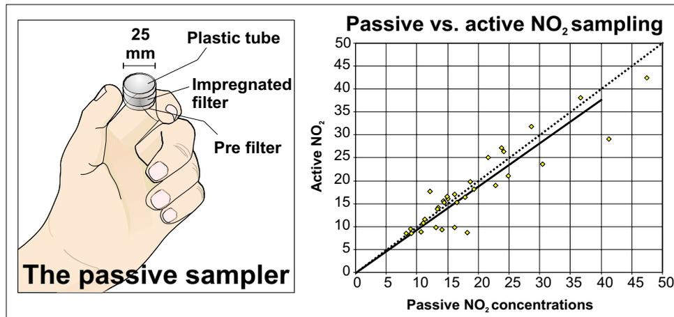
A sensitive diffusion sampler for sulphur dioxide (SO<sub>2</sub>) and nitrogen dioxide (NO<sub>2</sub>) developed by the Swedish Environmental Research Institute (IVL) and has been used in several investigations by NILU to undertake a screening of the spatial concentration distribution in ambient air.
