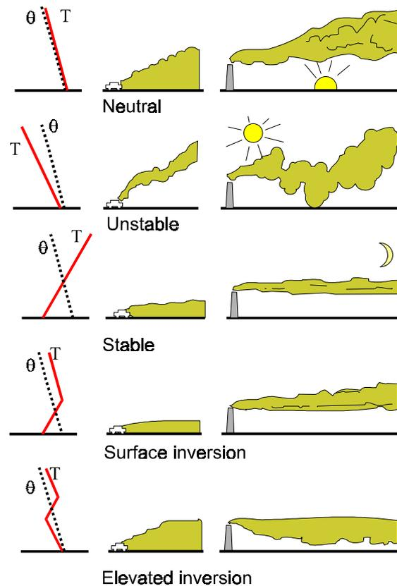
Figure 9.1: Schematic presentation of the atmospheric stability and the corresponding dilution of air pollutants above ground level.
