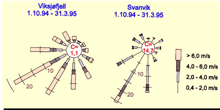
Figure 12.4: Wind roses for two different measurement sites; Viksjøfjell at a hill top (low friction), Svanvik in a valley (high surface roughness).
