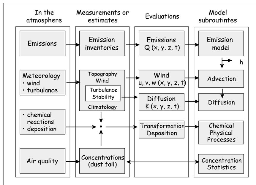
Figure 10.1: The procedure of an operational dispersion model used in practical applications.
