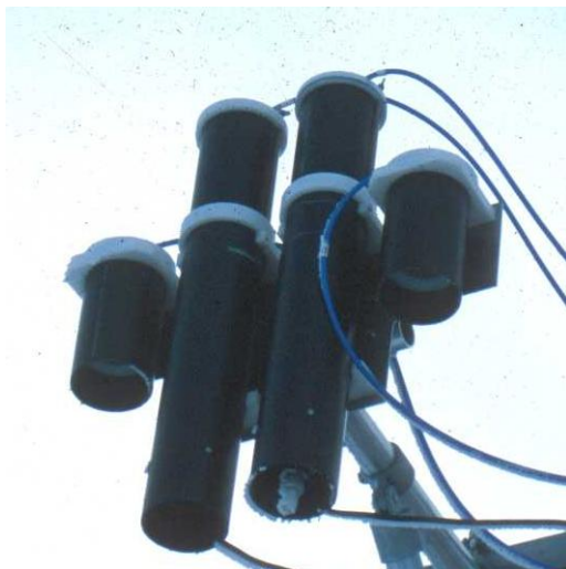
Figure A 4: Sampling of RGM and PM. Inside long tubes: Denuders for RGM sampling. Inside short tubes (separate and behind long tubes): Minitraps for PM sampling
